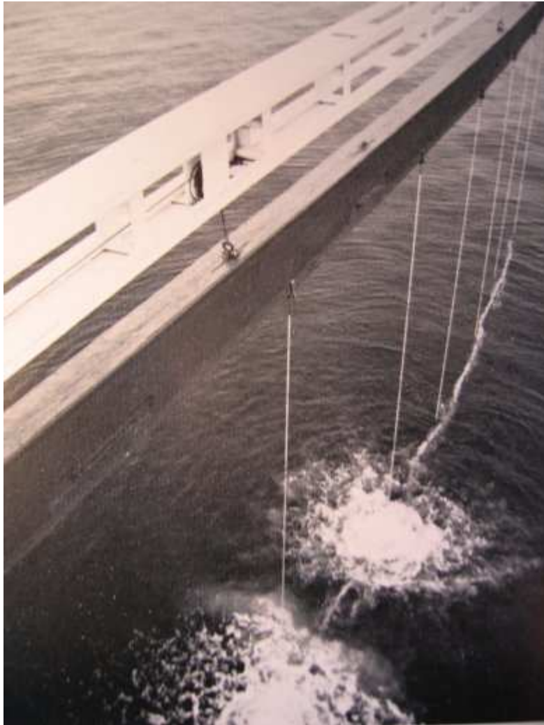
Figure 1: The shot-effect at close quarters revealing the direct disruption of the surface significantly before the bubble breaks the surface. Here the air evacuation of the furthest firing airgun can be clearly seen under the water whilst the shot effect on the surface is already well developed.
